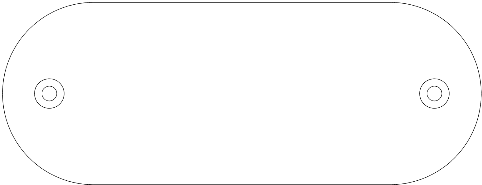
Side Panel make 1 - .125 thick cut profile .0625 deep
